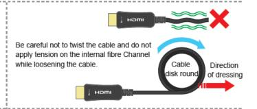
The HDMI connector cannot be suspended, the connector's junction will be deformed, and the internal fiber may be disconnected.
