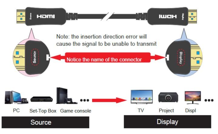
Source:Connect signal output device, such as Set top box, DVD, PC and Game console. Display:Connect signal input device; such as TV, Projector, Display.
